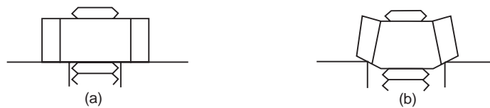
Figure 6.2 Schematic illustrating (a) proper nut seating and (b) improper nut seating due to an oversize bolt hole.
